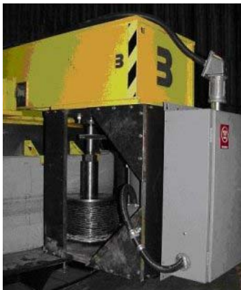
Figure 2 – Grinding unit attached to TPTA with one wheel-track of blades attached. 8-in. grind.
