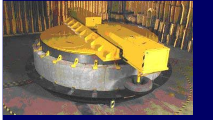
Figure 1 - Tire Pavement test apparatus at Purdue University.
