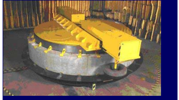
Figure 1 - Tire Pavement test apparatus at Purdue University.
