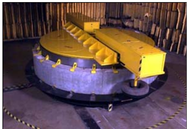
Photo depicts the SQDH's noise tester. The machine measures noise levels by running a tire over a concrete sample. Up to six different samples can be tested simultaneously.
