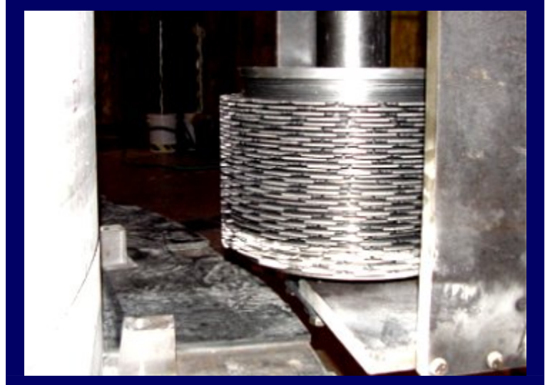
A close-up view of the grinding unit shows this specially designed and constructed equipment, which can grind two 8-in. wheel paths at the same time.
