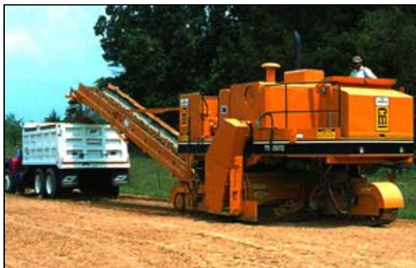
Photo of a subgrade trimmer. The machine trims the compacted subgrade to tight tolerances while using a stringline for guidance.
