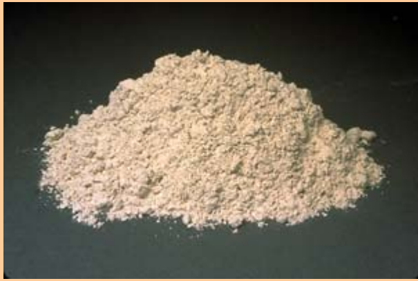
Slag cement is commonly referred to as ground granulated blast-furnace slag (GGBF).
